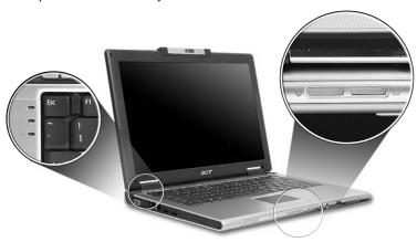
The front panel indicators are visible even when the computer cover is closed up.
